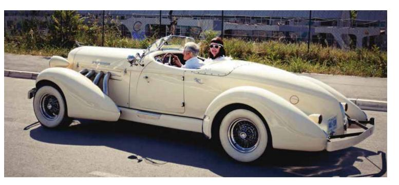
he Auburn 851 Speedster of 1935 was styled by designer Gordon Buehrig. The audacious 1935–1936 Auburn speedsters boasted curvaceous "boat-tail" bodywork on a potent supercharged eight-cylinder chassis, with a two-speed rear axle for relaxed highway cruising. A perfect storm of engineering and beauty, these cars combine elegance and modern drivability into an outstanding touring machine. The model has been referred to as the one genuine American
